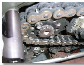
procket drift from the second retainer failure
