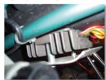
Side view of the cover shows the aluminum tubing I used to give the cover some stand off from the fins to promote air flow. Black lines were to mark where to bend and drill.
