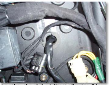
Grommet has now been added to protect the wiring. Those of you will sharp eyes will note I need to find a bigger grommet.
