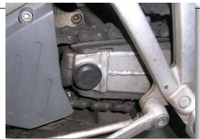
The misaligned chain with the chain guide on the swingarm
