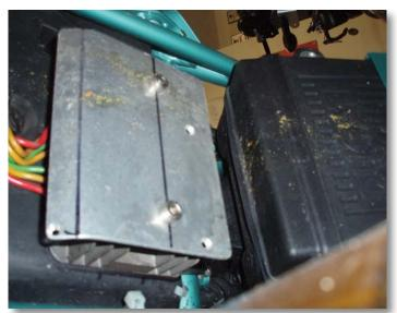
Second try with cover plate to protect the regulator fins. You can see some of the debris on the cover. Extra holes are there because I used some scrap aluminum I had lying around.
