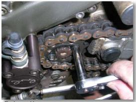
cheaper than the OEM retainer, is easier to get at an auto parts store, and will not rock back-and-forth in the same location and wear as quickly as the OEM retainer.
