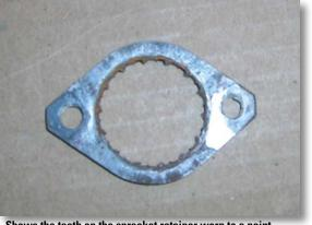
Shows the teeth on the sprocket retainer worn to a poin
