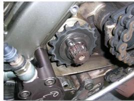
Worn sprocket pushed as close to the case as possibl
