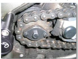
led attempt at using the end of the output shaft to hold the sprocket in place
