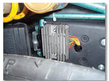
First try with the regulator under the seat pan. Wire routing is easy to see.
