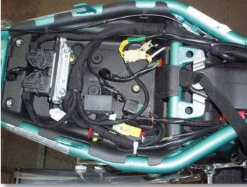
First try top view with wire routing. Notice the brass capture nuts that have the regulator bolts coming up from the bottom.
